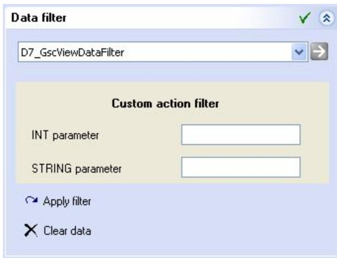
To achieve the nested display, the additional callback functions of the structure `TPluginFilterDefinition` have to be implemented. The Borland Delphi © example "GSCViewDataFilter" demonstrates the details.
